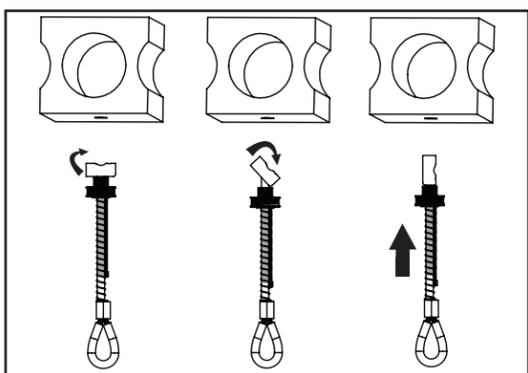
**2.** Rotate toggle bar into open position and insert into hole.
