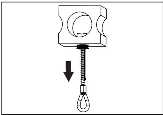
**4.** Pull on anchor loop and ensure toggle bar is fully seated in locked position as seen in the **TOGGLE POSITION DIAGRAM**. The hole plug should be fully seated in drilled hole.
