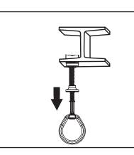
4. Pull on anchor loop and ensure toggle bar is fully seated in locked position as seen in the **TOGGLE** POSITION DIAGRAM. The hole plug should be fully seated in drilled hole.
