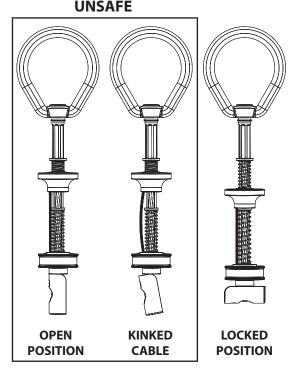
The Trigger and Trigger-wire may be used as a means of determining toggle position when view of toggle bar is obstructed by the anchorage. Trigger should be in contact with the trigger stop washer AND Trigger-wire should be straight in-line with the rest of the device to ensure toggle bar is in locked position.
