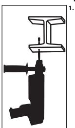
1. Drill a 11/16" (18mm) hole in the steel flange. Steel thickness must be between .25" (6.4mm) and 1.25" (31.75mm). Hole should be no closer than 1.5" (38mm) to any edge.
