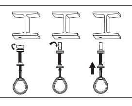
2. Rotate toggle bar into open position and insert into hole.
